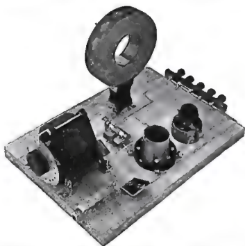
HOW THE SIMPLE LONG-WAVE RECEIVER LOOKS WHEN BUILT ON A "BREADBOARD"
